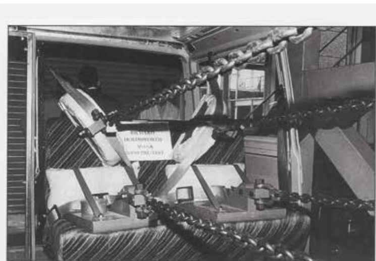
Ready to take the strain — bolsters in position, standard seat belts replaced by heavy-duty versions, each chain connected to a hydraulic ram.
