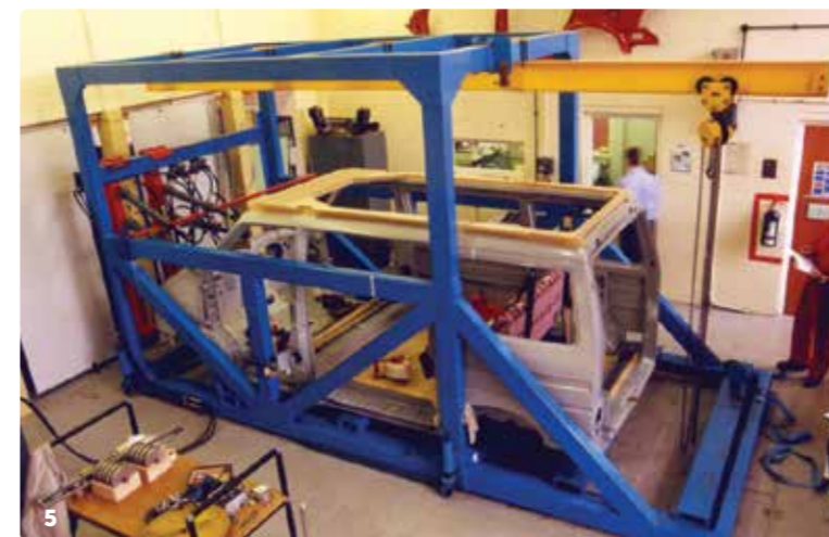
5: This is the serious stuff! A "pull" test at the Motor Industry Research Establishment with a Volkswagen "shell" proved that Holdsworth engineers had done their homework.
